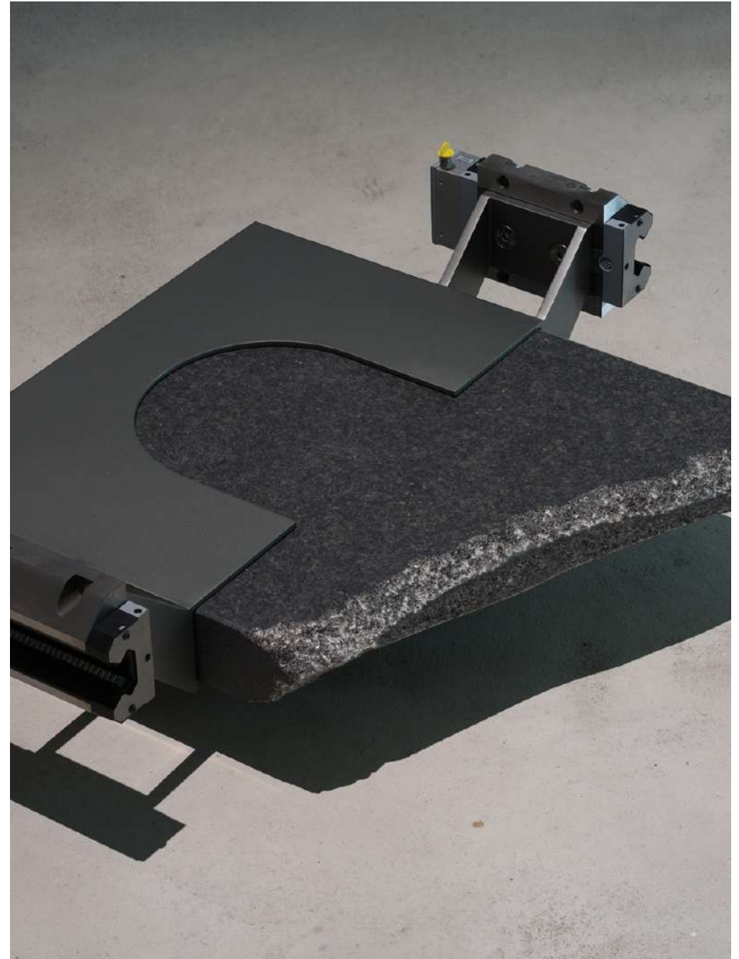
Richtebene, 2024, granite [DIN876/0], S355MC, linearguide, 785 mm x 605 mm x 230 mm
